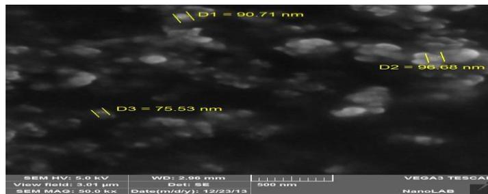
Figure 4: Scanning electron microscope of zirconium silicate nano-powder.
