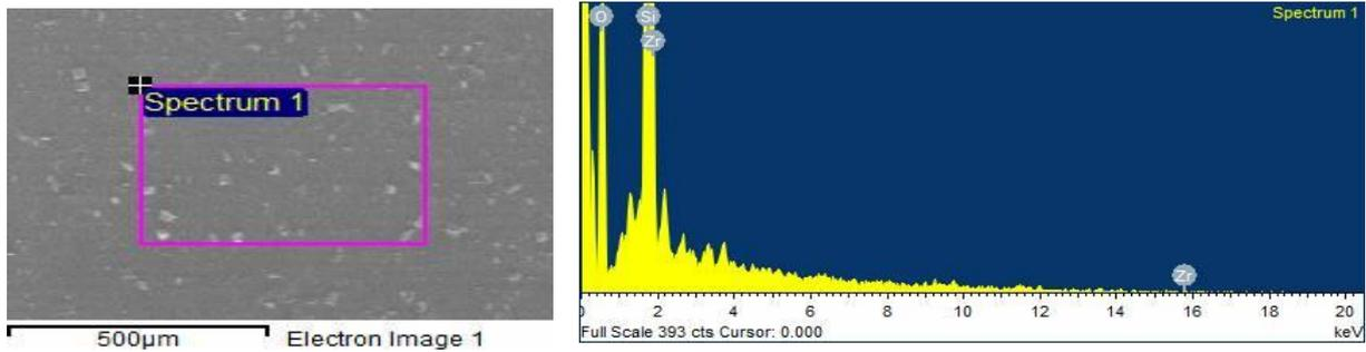
Figure 6: Energy Dispersive Spectroscopy to sample of silicone/nanocomposite showing peaks of (O, Si, Zr) elements
